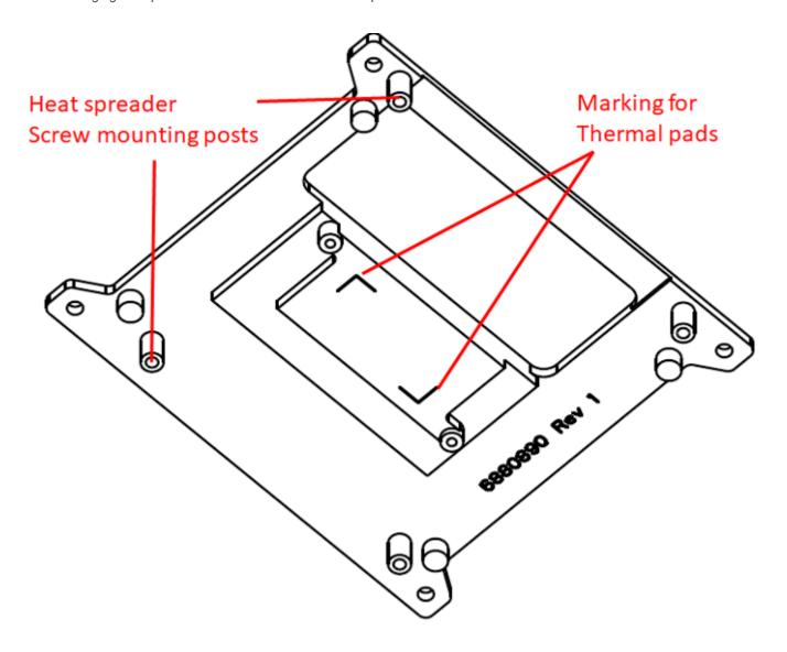
Heatspreader bottom view Take care not to damage thermal pads.
