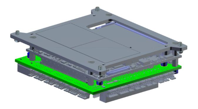
3D view of Gemini assembly with heatspreader
