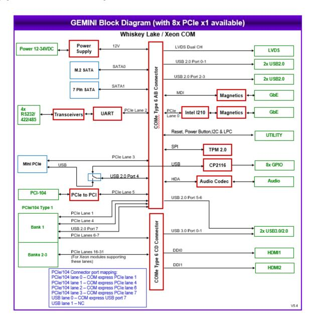
Gemini without PCIe Switch Block Diagram
